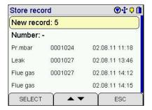
Open the "Selecting and entering customer data" function using (SELECT). This function enables editing the customer data shown, selecting another customer or creating a new customer.
