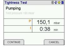
If the pressure reached the test pressure, the internal pump is automatically stopped.
