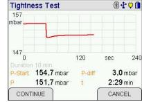
The start and stop values as well as the up to 20 intermediate measurements and the elapsed time were retained. These retained values can be stored and transferred to a PC at a later point in time. Measurement reports, which show the chronological sequence of the measurement in a diagram, can be printed using the PC200P software.
