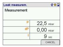
If the pressure in the gas pipeline to be tested has dropped by more than 0.9 hPa (mbar) or if the measurement takes longer than 5 minutes, the internal magnetic valve is opened and gas from the gas pipeline can flow through the comparison leak.
