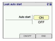
The measuring device recognizes a drop in pressure and automatically starts the leak rate measurement.
