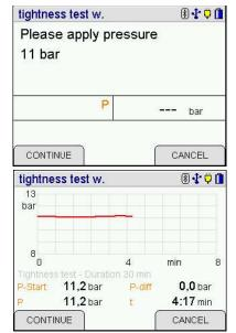
At the end of the measurement or after manual termination, a switch to the result display occurs and the documentation menu can be accessed.
